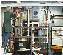
CSIRO/SRL Plasma test Rig used for the destruction of ozone depleting substance
